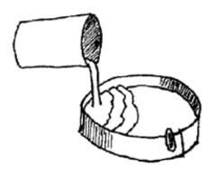
track with plaster. Pour it relatively thick to make a good strong cast. This is the time to add and reinforcing materials such as string, wire, or twigs. Once you have finished pouring, let the track set for at least 1/2 hour. Some types of plaster may take longer to set.
